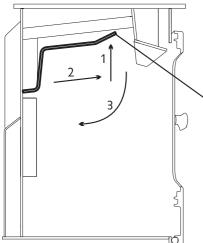
Lift throat plate at front, then pull forward and swing down.
