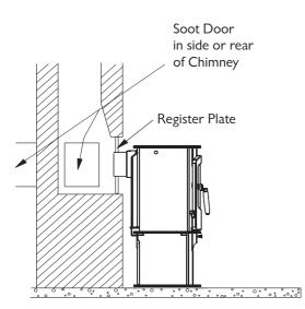
Fig. 7. Horizontal register plate with rear flue connection
