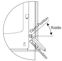
Door Opening Tool rotated 180° and pushed fully on to Riddler Knob
